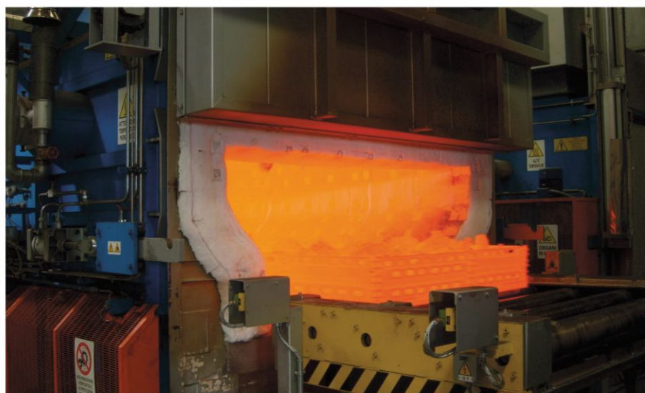
▲ Continuous Roller Hearth Heat treatment furnace in Gas fired heating
